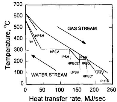
**Fig. 2** Heat transfer rate-temperature diagram of the triple pressure HRSG (case III)
